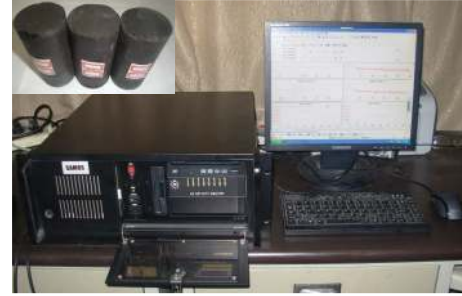
FIGURE 1: Coal samples and acoustic emission system.
