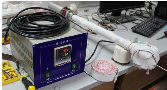
Figure 8. Annealing the copper rod of the HPGe using the heating ingot, asbestos belt is added to prevent the heat loss.
