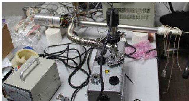
Figure 7. The copper rod of the HPGe cold finger is annealing using heating belt.
