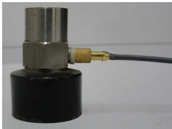
Fig. 9.5 Accelerometer (Contacting type magnetic probe)
