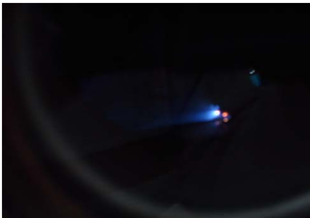
Fig. 4: Fluorescent image for higher applied voltage and the emitted current was recorded to be \sim 45 micro amperes
