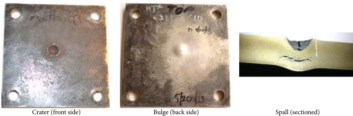
FIGURE 5: Typical target plate after an experiment.
