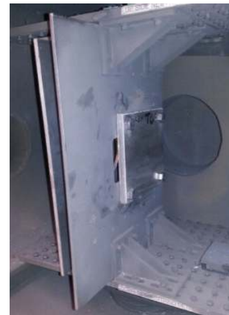
FIGURE 2: Target plate bolted inside the gas gun chamber.
