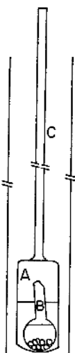
Figure 1. Calorimetric cell: (A) an outer cell; (B) an inner cell; (C) glass rod.
