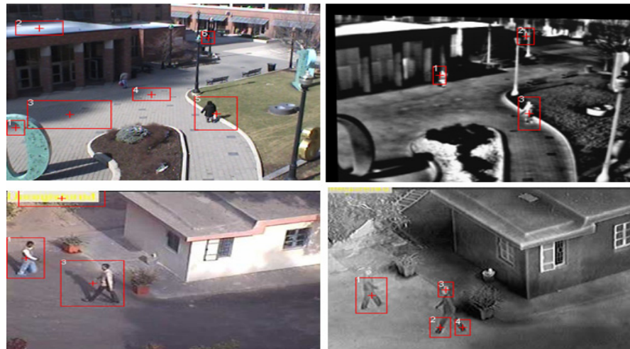
Figure 7: Visible and corresponding thermal infrared in a) Variable illumination due to cloud movement causing false detection in visible (top) b) Incorrect detection due to shadows in visible and thermally insulated clothing in infrared (bottom)
