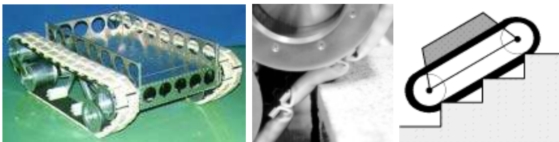
(a) XEVIUS tracks (b) XEVIUS track close up (c) XEVIUS track principle
