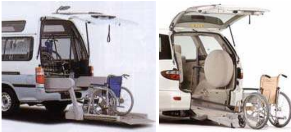
(a) Wheelchair lifter platform
