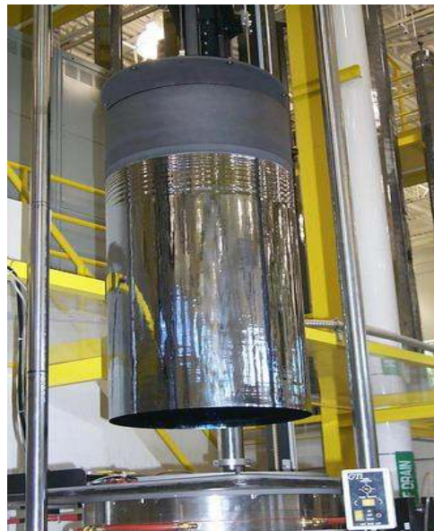
(b) Photograph of Large thin-walled cylinders grown by EFG process.
