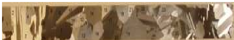
Figure 5.11 A photograph of a silicon beam with labeled grains prepared for x-ray diffraction.
