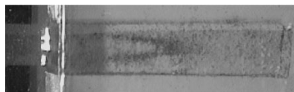
Fig. 10. Photograph of liquid streaming in U-type liquid cell 90 s after SAW is generated. The sample is 60 wt % glycerol/water mixture.
