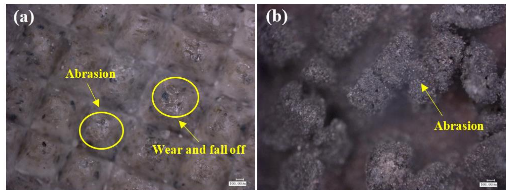
Figure 16. (a) shows 3M abrasive belt grit, (b) shows VSM abrasive belt grit.
