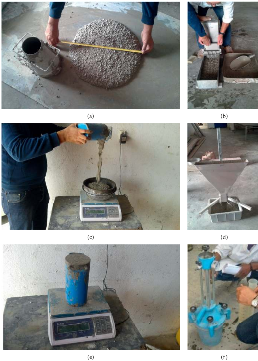
FIGURE 3: Test on the four SCCs in the fresh state. (a) Slump flow test. (b) L-box test. (c) Sieve stability test. (d) V-funnel test. (e) Bulk density. (f) Air content test.
