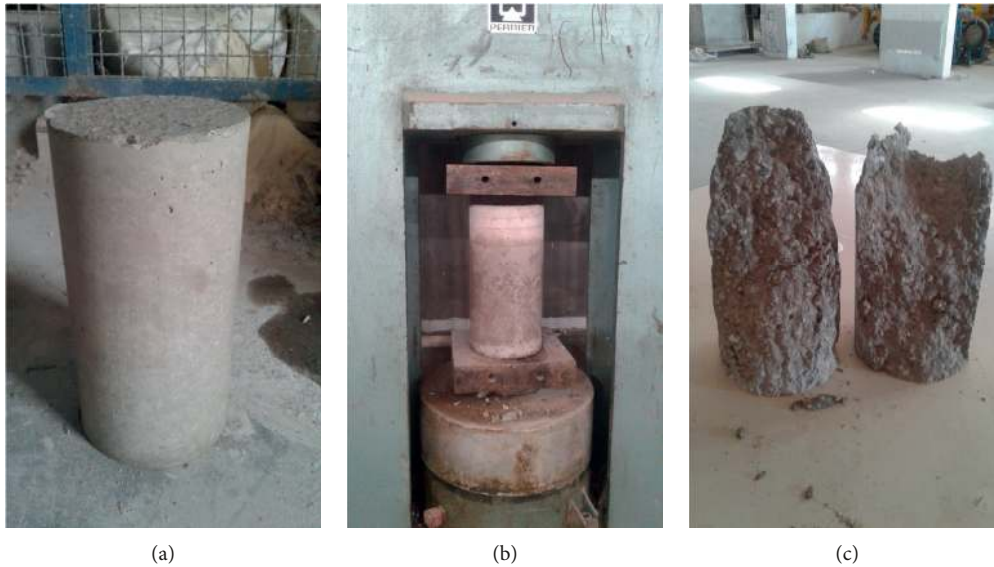
FIGURE 5: Compressive strength test.
