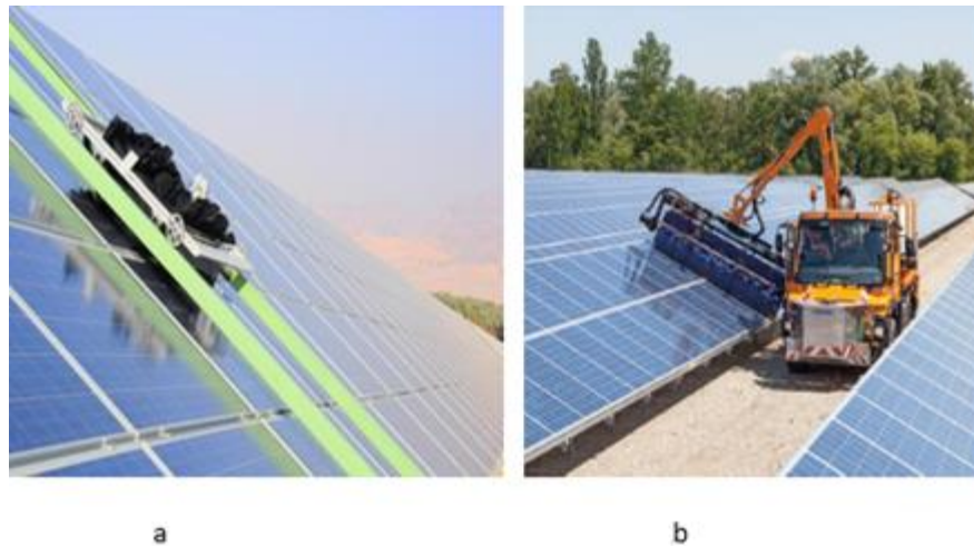
Figure 2. (a) Waterless cleaning of solar panels via robot and b) FWG panel washer.
