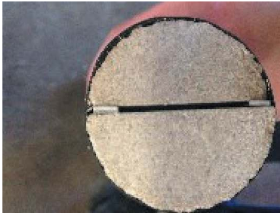
Fig. 7. Fracture in the limestone core
