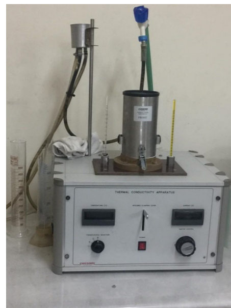
Fig. 5 Thermal conductivity Test device
