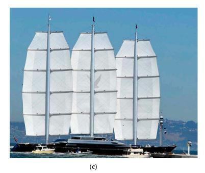
**Figure 12.** The three mainstream WASPs on board: (a) Flettner rotor (Courtesy of Alan Jamieson) (CC BY 2.0); (b) Towing kite (Photo reproduced with permission; copyright SkySail Group); (c) Soft sail (The Maltese Falcon) adapted from lj16/Wikipedia (https://commons.wikimedia.org/wiki/File: The\_Maltese\_Falcon\_(2906785674).jpg) (CC BY) accessed on 5 January 2022.
