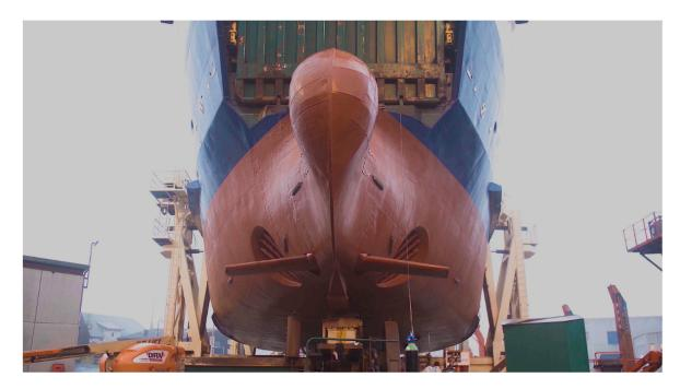
**Figure 7.** Wavefoil's retractable bow foil installed on ferry, M/F Teistin (Photo reproduced with permission; copyright Wavefoil).
