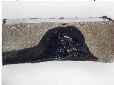
(c) the cross-section of molten pool when burn-through occurs
