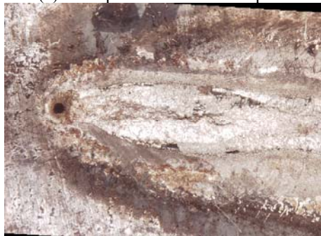
(b) the back surface of molten pool
