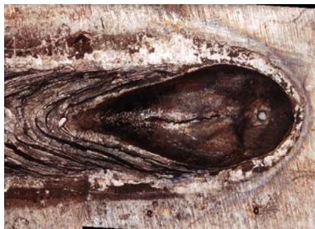
(a) the top surface of molten pool
