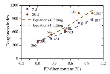
Figure 9. Relationship between toughness index and PP-fiber content.
