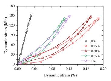
**Figure 15.** Hysteresis loops of FCIT at different PP-fiber contents (N = 500).
