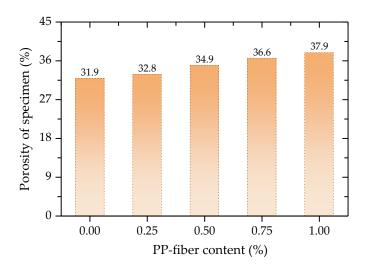
Figure 18. Porosity of specimen at different fiber contents.
