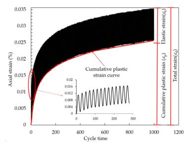
Figure 19. Strain curves with increasing cycle time.
