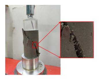
Figure 10. Damaged surface of specimen.
