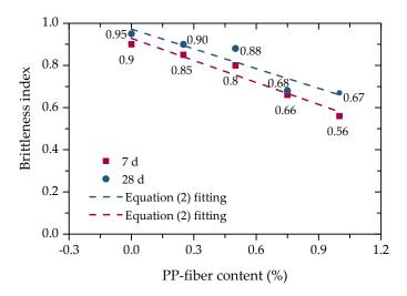
Figure 8. Relationship between brittleness index and PP-fiber content.
