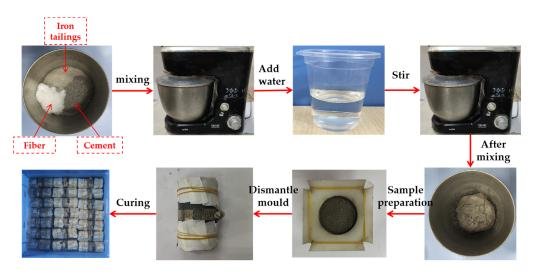
Figure 2. Sample preparation flow.
