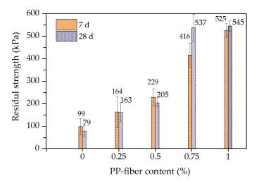
Figure 7. Residual strengths of FCIT at different curing ages.
