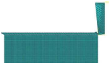
FIGURE 4: Finite element model of wheel tread reprofiling.
