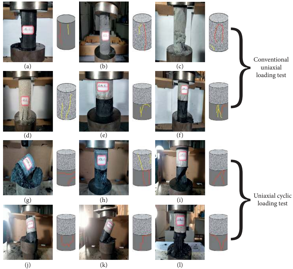
FIGURE 4: Test results and the failure modes of samples: (a) M1-1, (b) NY-1, (c) XS-1, (d) ZS-1, (e) XSM1-1, (f) ZSM2-2, (g) NYM1-3, (h) NYM1-4, (i) XSM1-3, (j) XSM1-4, (k) ZSM2-6, (l) ZSM2-7 (in the figure, the yellow line indicates the position of the crack after the failure of the sample, and the red line represents the boundary of the spalling area of the sample).
