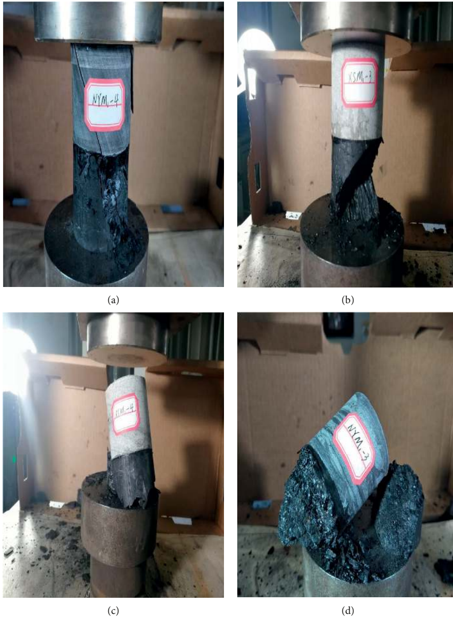
FIGURE 11: Failure characteristics of cyclic loading of samples. (a) Four cycles. (b) Seven cycles. (c) Eight cycles. (d) Ten cycles.
