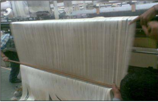
Figure 14. Damaged warp yarns is dragged out
