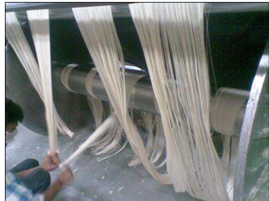
Figure 28. Damaged warp yarns are cut
