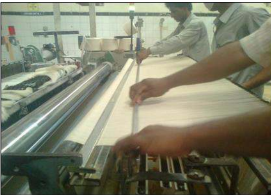
Figure 15. Dressing of new warp yarns
