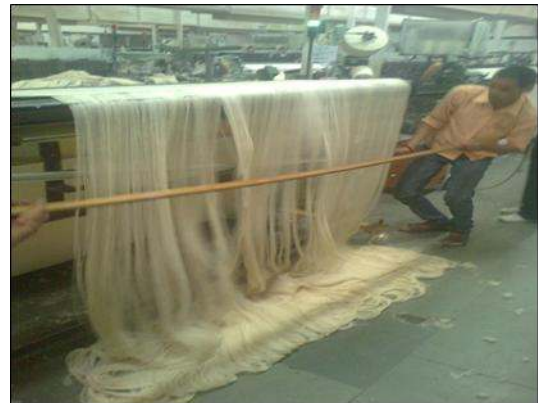
Figure 25. Crossing damaged ends are taken out before knotting process
