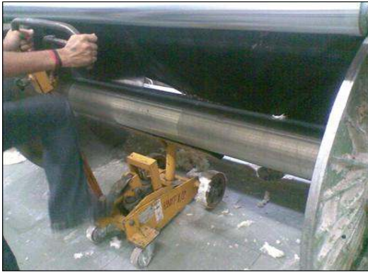
Figure 9. Unloading of empty beam
