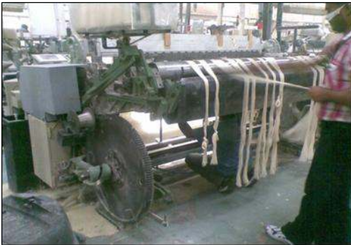
Figure 10. Dressing of warp yarns
