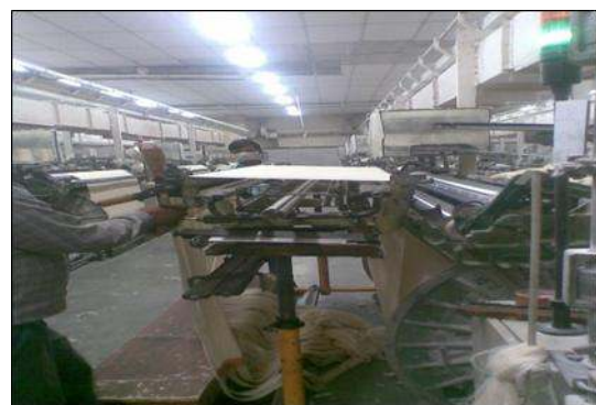
Figure 13. Warp sheet is pulled out from new beam
