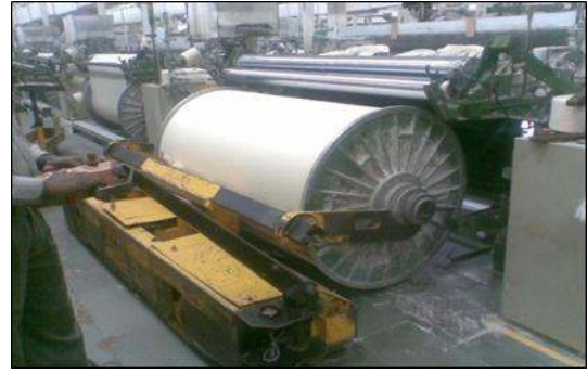
Figure 11. Loading of the new sized beam
