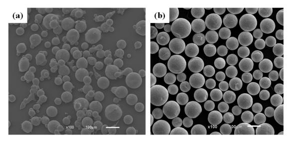
Figure 1. SEM images of (a) Ni60A powder and (b) WCPs.
