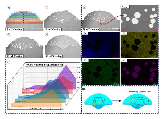
**Figure 3.** (a) The cross-sectional morphologies of coating of 0 mT; (b) the cross-sectional morphologies of coating of 10 mT; (c) the cross-sectional morphologies and the element map of Cr, Fe, Ni, W of coating of 20 mT; (d) the cross-sectional morphologies of coating of 30 mT; (e) the cross-sectional morphologies of coating of 40 mT; (f) the WCP proportions in particle volume ranges of coatings; (g) schematic diagram of the evolution mechanism of the WCP distribution.
