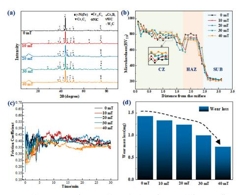
Figure 5. (a) XRD patterns of coatings; (b) microhardness of coatings; (c) friction coefficient curves of coatings; (d) wear mass loss of coatings.
