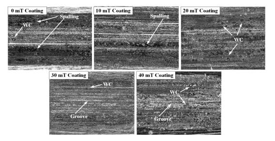
Figure 6. The wear morphology of the coatings.
