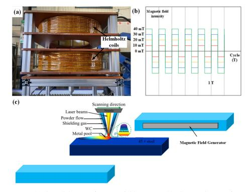
**Figure 2.** (a) Physical diagram of magnetic field generator; (b) schematic diagram of magnetic field waveform; (c) experimental schematic.
