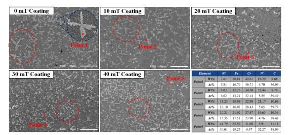
**Figure 4.** SEM images of middle regions of coatings and element composition at different points on the surface of coatings.
