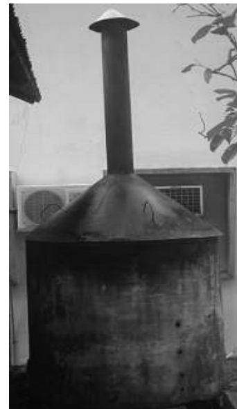
Figure 1. The ferro-cement furnace.
