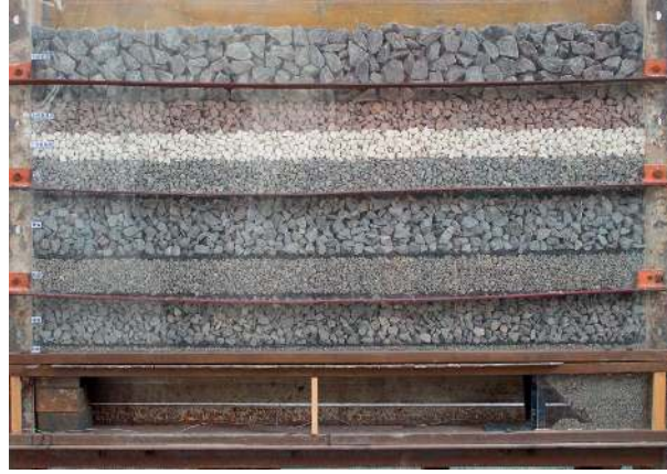
FIGURE 11: Overview of the experimental model of complex structure coal seam.
