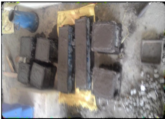
Figure 1: Casting of specimen
