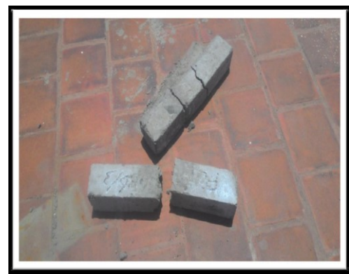
Figure 8: Flexural strength test before breaking due to self-weight.
