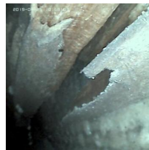
(f) Splitting of the wood keel
