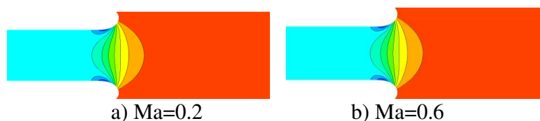
Figure 7. Static pressure distribution contours on the longitudinal section (different outlet Ma Number)
