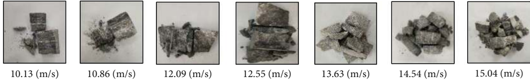
FIGURE 3: Damage pattern of pomegranate biotite schist at different impact velocities.
