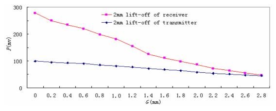
Fig.6 results of 2mm lift-off for transducers
