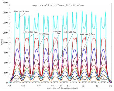
Fig.2 The calculation results of the induced magnetic field distribution
