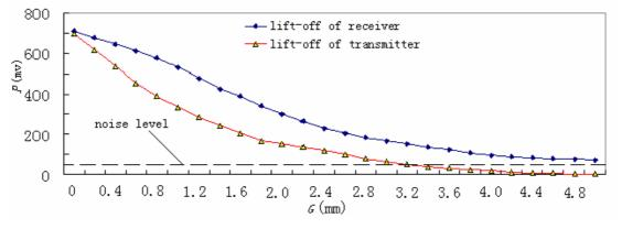
Fig.5 received signal at different lift-off values of transducers Keeping the lift-off of transmitter and receiver 2mm individually, and increasing the lift-off of the other, the results are shown in Fig.6. It is concluded that 2mm lift-off of transmitter is more stable, and the signal changes little no matter the lift-off of the receiver. So in order to make the transducers work stably in complex environment, the
