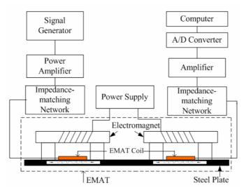
Fig. 4 block diagram of the experimental setup
