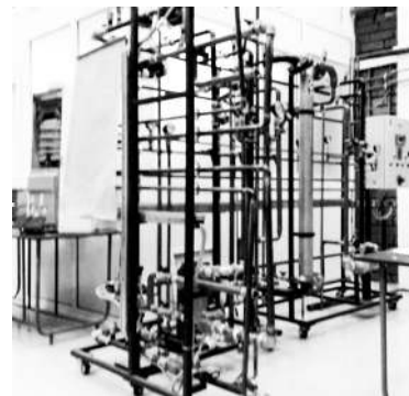
Fig. 6 Heat exchanger testing stand
