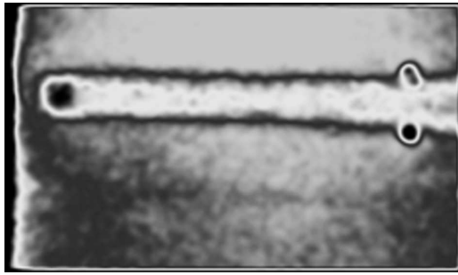
Fig. 4. IR thermogram of the PW-5 rudder.
