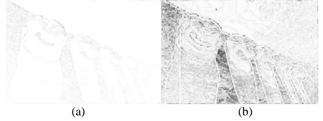
Fig. 2. Illustration of the distortion map calculated for a JPEG compressed image (bit rate 0.41bbp) with its original shown in Fig 1(a): (a) distortion map of PSNR, and (b) distortion map of SSIM. The lower the intensity, the larger the distortion is.
