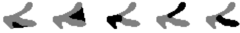
Figure 2: Cavities (left two images) and parts (right three images) for alaph. The potential cavity at the top of the letter is rejected because its thinness makes it potentially unstable.
