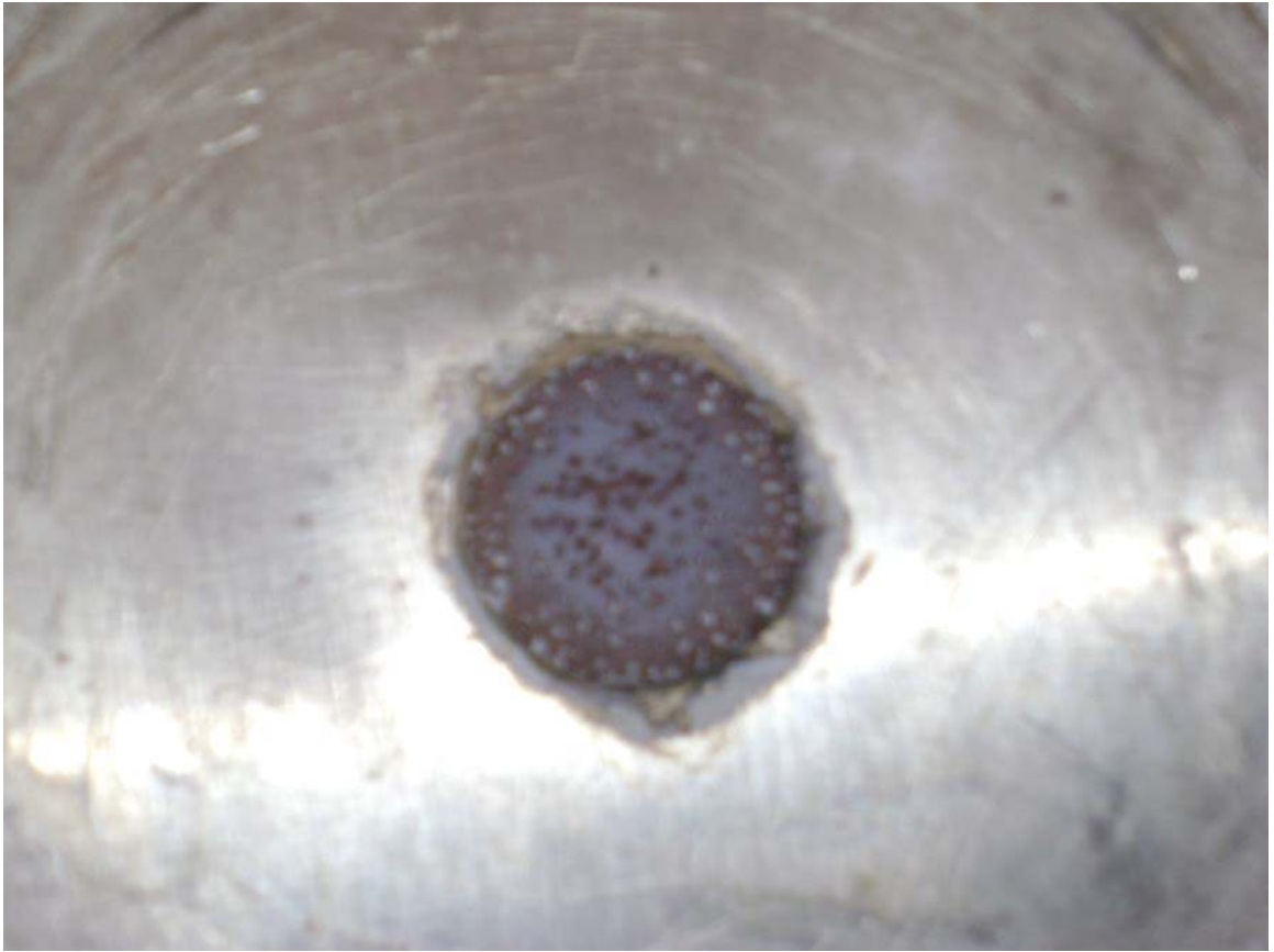
Figure D: Copper Hat after 0.4% wt Nanofluid Experiment
