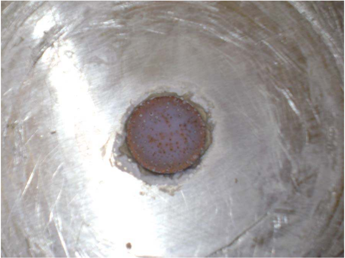
Figure C: Copper Hat after 0.3% wt Nanofluid Experiment
