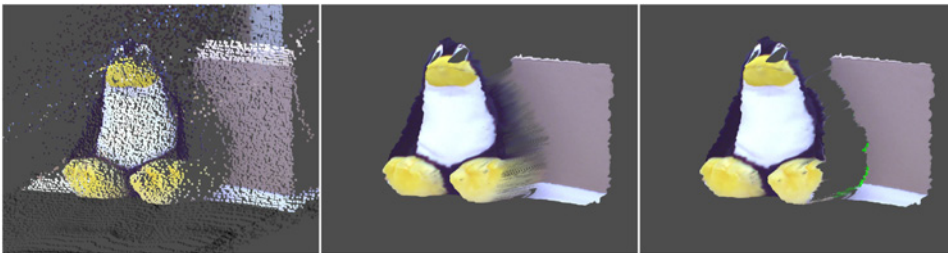
Figure 9 Results of combined refinement and 2D/3D data for a 160 \times 120 PMD sensor (upscale factor 8): (a) Raw input data; (b) Biquadratic refinement; (c) our approach (green pixels indicate occlusions).
