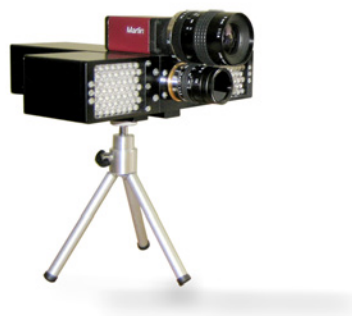
Figure 2 2D/3D camera setup consisting of a 19k PMD and a high-resolution CCD-camera mounted on top.
