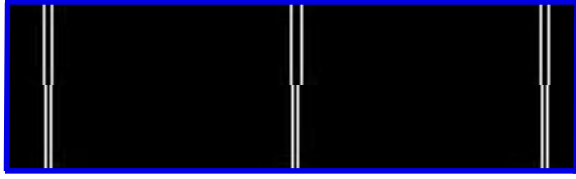
Fig. 3: Composite image with Canny edge detection (upper image) and Sobel edge detector (lower image), computed over the same set of lines of the reticle shown in Fig. 1
