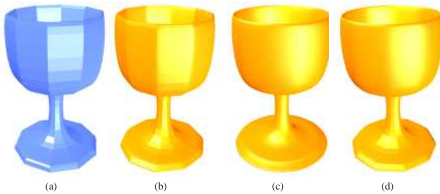
Figure 4. Interpolating surfaces with different shape parameters using two-phase scheme for Doo-Sabin subdivision: (a) given mesh; (b) interpolating surface with all shape parameters set to 0.85; (c) interpolating surface with all shape parameters set to 0.4; (d) interpolating surface with local shape control: shape parameters of the bottom part set to 0.85 and others to 0.4.
