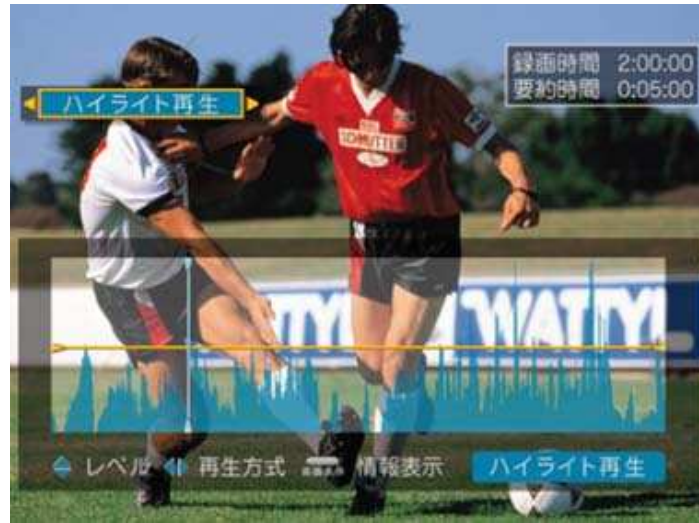
Figure 2: A screenshot from the Mitsubishi Electric “Raku-reko” DVD Recorder. This interface uses summarization during playback of a recorded sports program, allowing the user to view only the exciting portions of the program.
