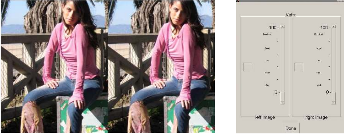
Figure 3: Graphical user interface for the DSCQS methodology adapted to high resolution images.
