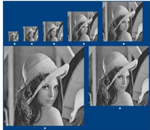
Fig. 5. Test images for the relative perceived quality assessment test (“Lena” coded by JPEG 2000 at 0.1 bits/pixel).
