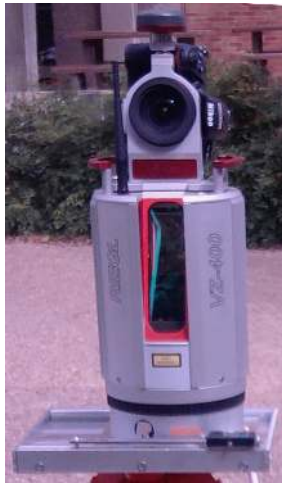
Fig. 2. The RIEGL VZ-400 terrestrial range scanner and co-registered Nikon D7 00 DSLR camera used to collect stereoscopic signals.
