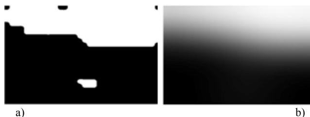
Figure 7: a) Fusion mask obtained from section 2.2.2. b) Fusion mask with blurred with a Gaussian kernel
