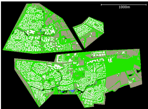
Figure 3. AHN3 point clouds used in this work. The upper left part shows the training set, the upper right part shows the validation set and on the bottom is the testing area. Green: unassigned; brown-gray: ground; white: buildings; blue: water; red: bridges.
