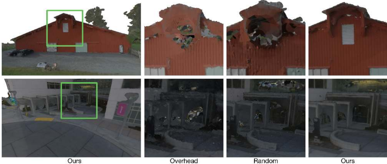
Figure 4. Qualitative comparison of the 3D reconstructions obtained from an overhead trajectory, a random trajectory, and our trajectory for two real-world scenes. Our reconstructions contain noticeably fewer visual artifacts than the baseline reconstructions. In all our experiments, we control for the flight time, battery consumption, number of images, and quality settings used in the 3D reconstruction.
