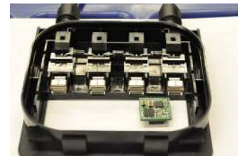
(b) Photograph showing discrete implementation of the power converter together with a solar panel junction box.
