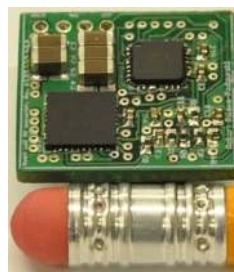
(a) Photograph of the sub-module MPPT converter with pencil shown for scale. The power inductor is on the bottom side of the PCB.
