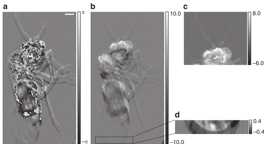
Figure 3 | Phase-contrast images of a fruit fly. (a) The GBH interferometer retrieves a phase-difference image of the fruit fly, which contains phase wraps in the body. It is the sum of two phase-shift images of opposite signs, with a vertical offset of 140\ \mu\text{m} . Scale bar, 200\ \mu\text{m} . (b) The unwrapped phase-difference image. (c) By a shift-and-sum algorithm, an absolute phase-shift image of the head portion of the fly was retrieved. The wingtip area outlined with a dotted rectangle in b is magnified in d and shown in a smaller grey scale. From the phase-shift values in this area, the thickness of the wing membrane could be estimated.
