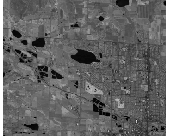
Fig. 1. Channel 75 (at an infrared wavelength of about 1.06\mu\text{m} ) of a 224-channel AVIRIS image taken near Denver, Colorado. This image is of size 614 \times 512 pixels, with each pixel corresponding to approximately 15m on the ground.
