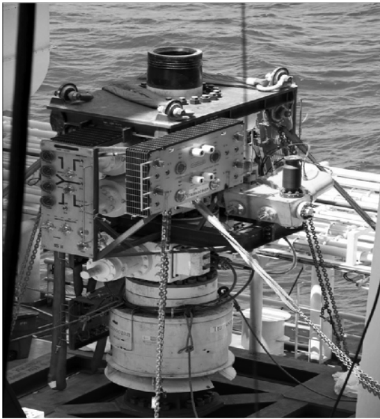
Fig. 5 Capping stack on drillship ready to be installed (source: BP)
