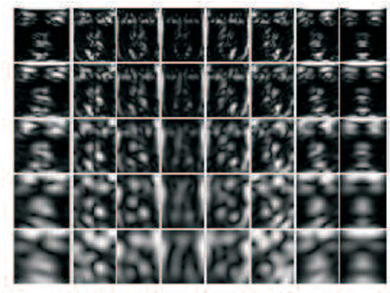
Fig. 14.6. The output of an image sample from the database convolved (filtered) with 40 Gabor filters (5 frequencies and 8 orientations).
