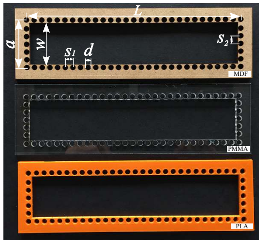
Fig. 5. Prototypes of Layer II of the [5.15-5.85] GHz AFSIW interconnection before assembly of Layers I-III. Optimized dimensions for all materials under study: a = 40.0 mm, w = 36.0 mm, L = 182.0 mm, s_1 = 6.5 mm, s_2 = 6.78 mm, and d = 4.0 mm. The thickness of Layer II is fixed to h_2 = 3.0 mm.
